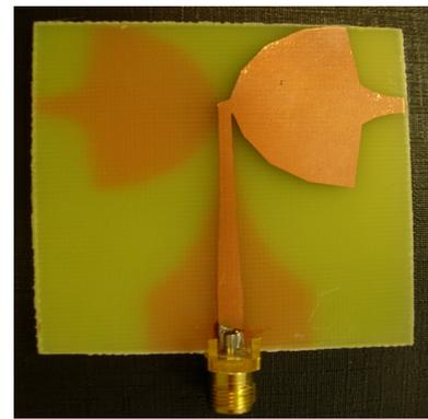
Fig. 6. CC-Parallel Strip Antenna in FR4 substrate
