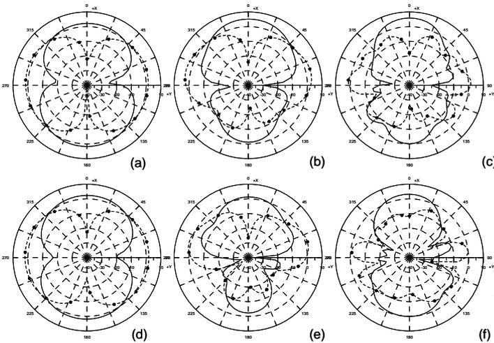
Fig. 5. H-plane copolar and crosspolar(dashed) field pattern (a) CC-PS at 3.1 GHz (b) at 6.85 GHz (c) at 10.6 GHz (d) EE-PS at 3.1 GHz (e) at 6.85 GHz (f) at 10.6 GHz
