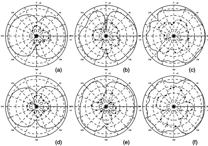
Fig. 4. E-plane copolar and crosspolar(dashed) field pattern (a) CC-PS at 3.1 GHz (b) at 6.85 GHz (c) at 10.6 GHz (d) EE-PS at 3.1 GHz (e) at 6.85 GHz (f) at 10.6 GHz
