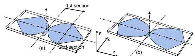
Fig. 1. Antenna geometries without balun. (a) CL-PS structure. (b) EL-PS structure
