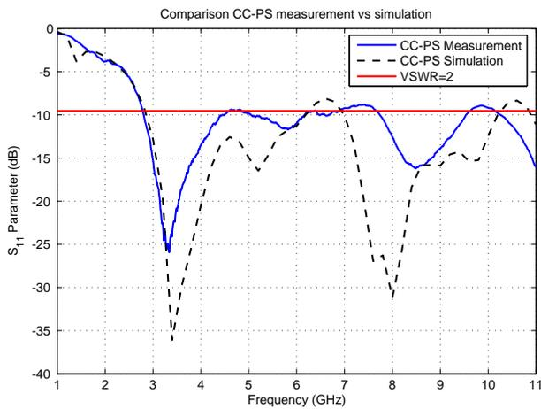
Fig. 8. CC-Parallel Strip Antenna simulation versus experimental results
