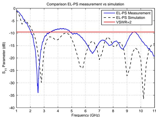
Fig. 9. EC-Parallel Strip Antenna simulation versus experimental results
