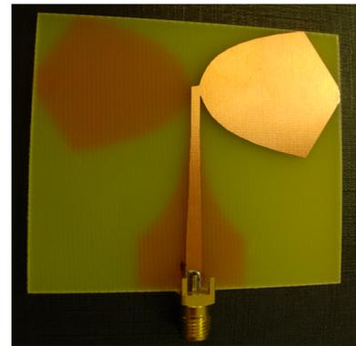
Fig. 7. EL-Parallel Strip Antenna in FR4 substrate
